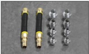
Allison Adapter Kit (optional) #40201346 Includes 2 each: Connection Hoses, -8 (1/2 JIC), -12 (3/4 JIC), -16 (1" JIC), -20 (1-1/4" JIC)
